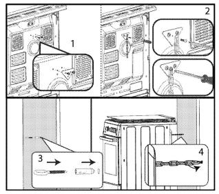
Stability chain to be as short as practicable to avoid oven tilting forward and diagonal to avoid oven side tilting.
